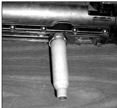
Soviet KPV Charging Handle Close-up
